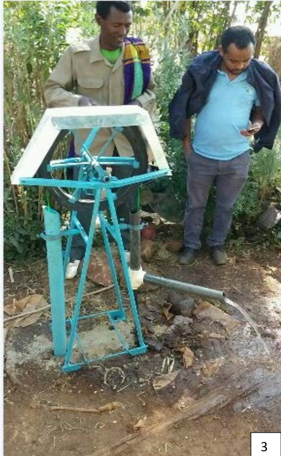
Rope and washer pump operated by hand
