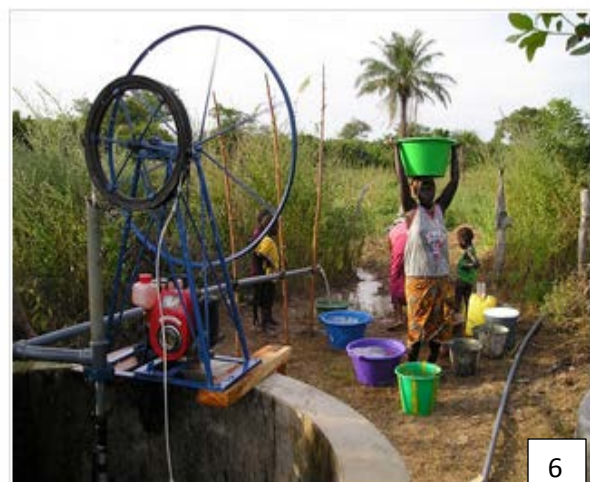
Rope and washer operated by motor
