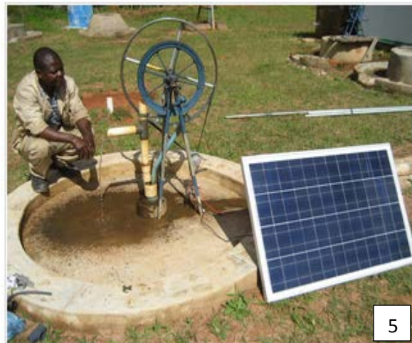
Rope and washer operated by solar energy
