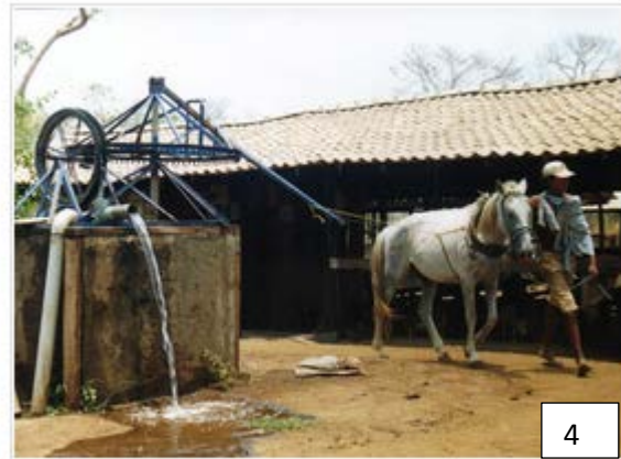
Rope and washer pump operated by a horse
