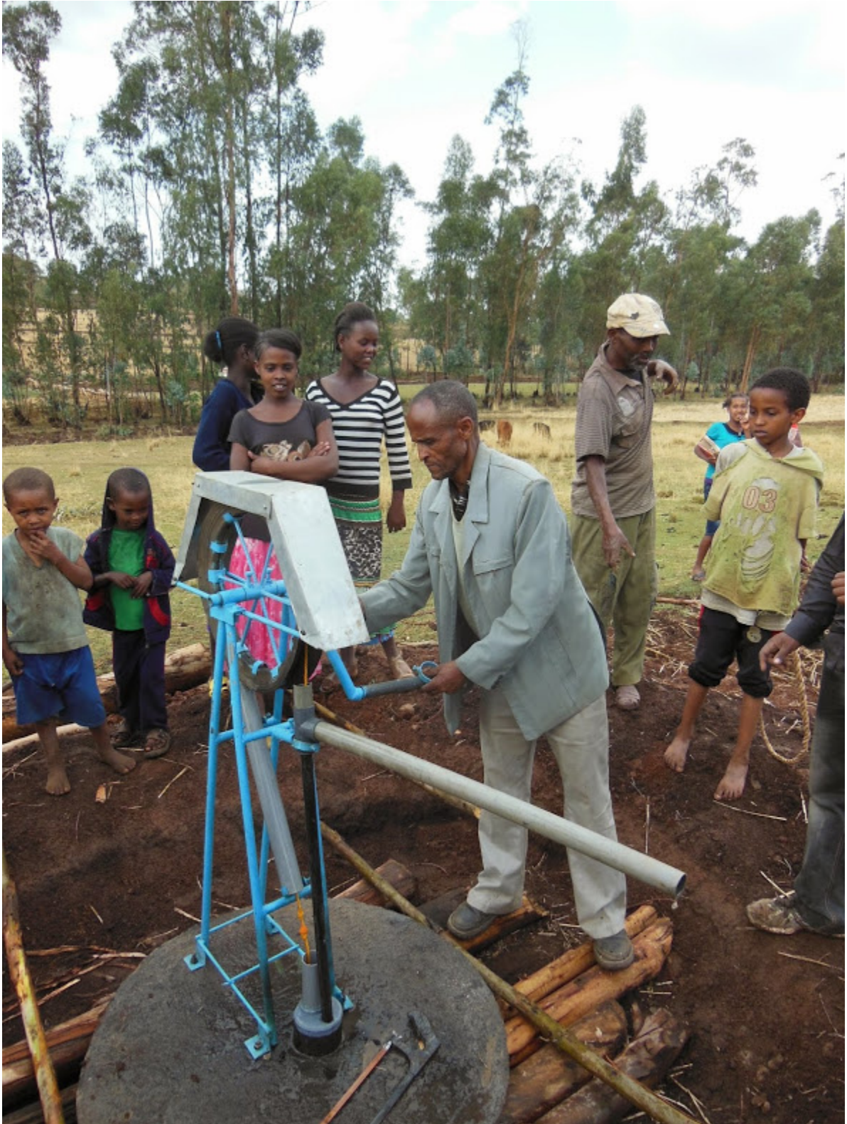
Rope and washer pump operated by hand
