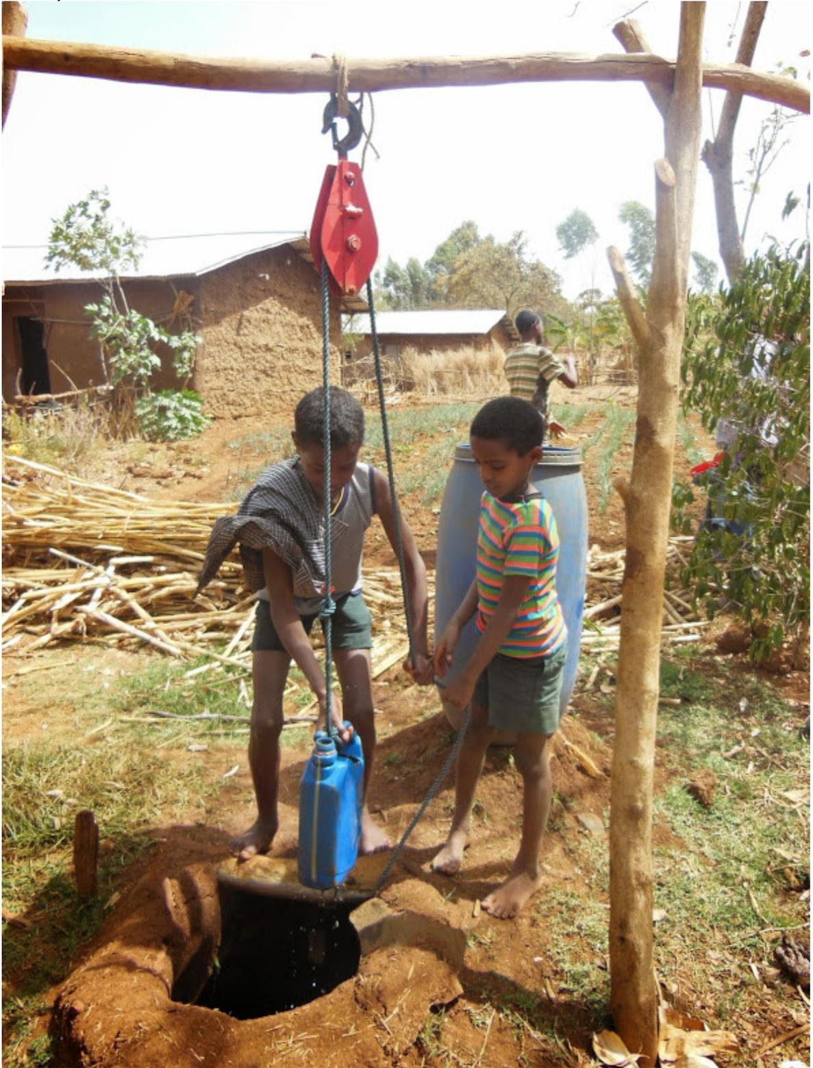
Rope and washer pump operated by hand
