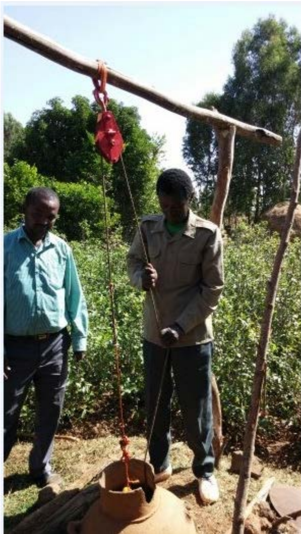
Pulley/Bucket system, Bahir Dar, Ethiopia
